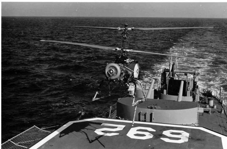
ASW torpedoes or a nuclear depth charge under its ribcage. In practice, the only authorized payloads were conventional warhead torpedoes. This was because the remote control technology and reliability of the DASH itself was suspect. Several DASH birds were lost in training exercises, as they mysteriously refused to respond to the flight controller's commands. One climbed vertically to around 30,000 feet on its own until it shook itself to pieces and
