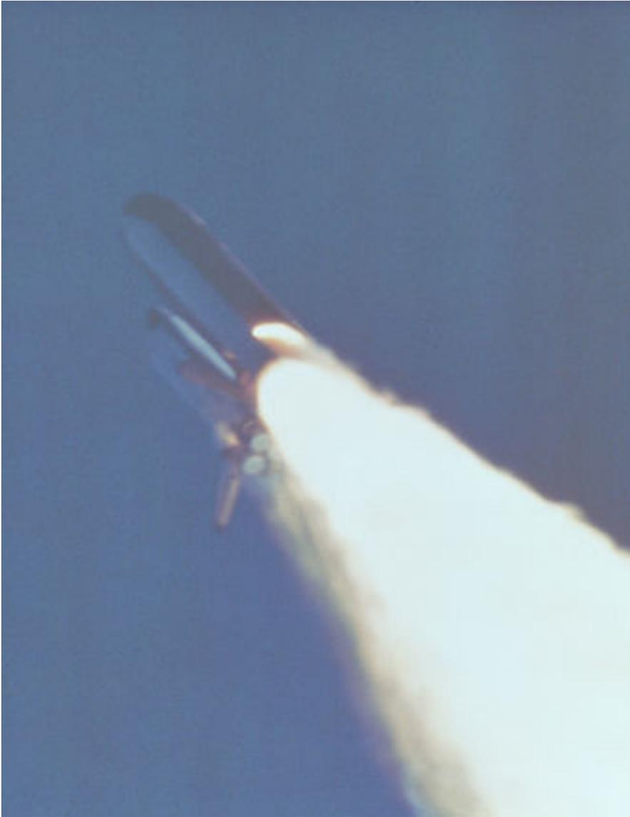
Finally the cause had been found and in my sorrow I could at least be thankful it wasn't my system that had caused the accident. Quickly it was determined that the cold weather had hardened an o-ring in one of the solid rocket joints. It didn't seal and the leak occurred.
