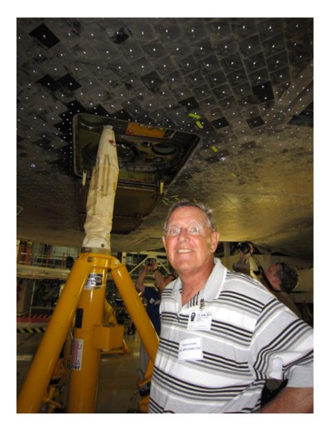
This story concerns the smaller valve to the left in the photo. It is known as the Gaseous Oxygen two inch disconnect and its purpose is to direct high temperature, high pressure gas at 400 psig from the Space Shuttle Main Engines (SSME) to the top of the Liquid Oxygen tank to pressurize the LOX tank during flight. Here's a schematic of the two inch disconnect.
